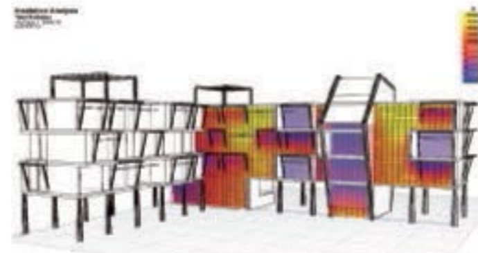
solar radiation south facade
